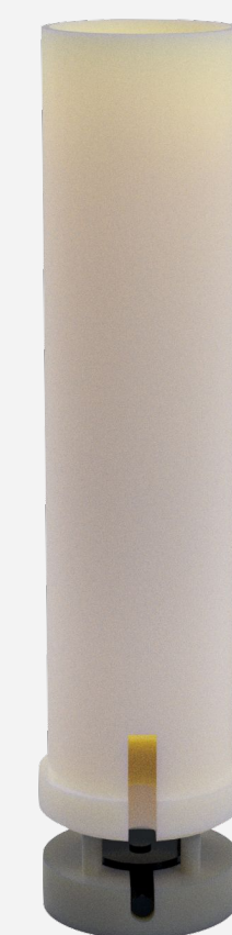
Figure 5: 3D printed disk to hold load cell
